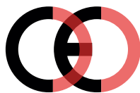
False CE Mark (too close)
